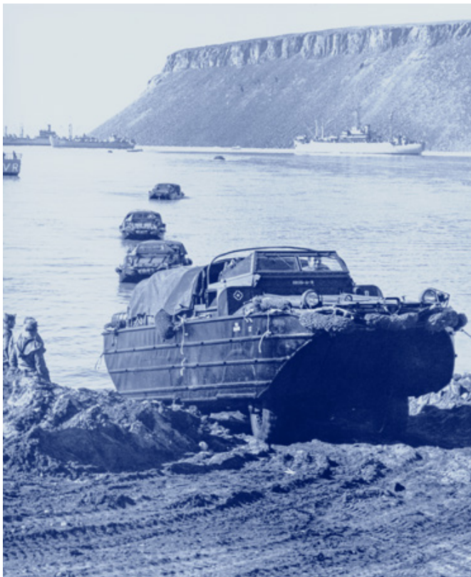
An amphibious truck, the DUKW, or “duck,” could easily carry two tons of cargo from a ship and then be driven up on shore for unloading.
